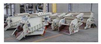
Thanks to high quality vibrating motors, they provide efficient feeding of very fine and coarse materials.
