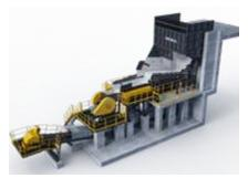
Hopper unloading, primary or secondary crushing stage (feeding of the crusher or screen)
